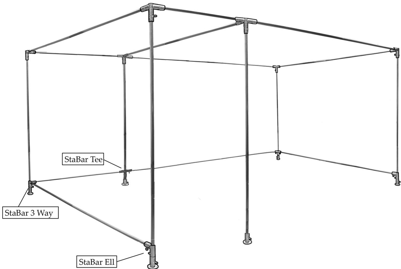
7. To complete your MeshPanel Booth Frame, insert remaining poles into StaBar Joints, clicking into place. Begin at the back of the booth, using a 116 ½" pole and a 57 ½" pole, then install the sides.
