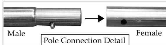
1. Connect male and female pole sections by clicking together to form (8) poles that are 116 1/2" long and (6) leg poles that are 82 1/2" long.
