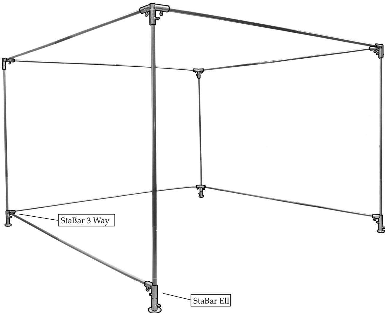
7. To complete your MeshPanel Booth Frame, insert remaining poles into StaBar Joints, clicking into place. Begin at the back of the booth, then install the sides.
